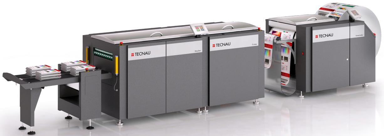
*The Stack 2320 cutting and stacking solution for color printers includes the Buffer 530, Cutter c23, and the Stacker s20.*
